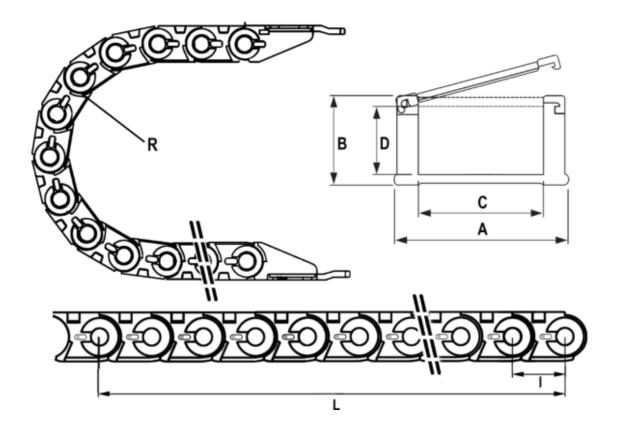
Full length = 990mm Inside Height = 23 Inside Width = 47 Link Length(Pitch) = 33 Outside Height = 31 Outside Width = 63 Radius = 035
